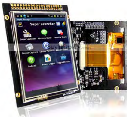
ER-TFTM032-3 with Resistive Touch Panel ↑
